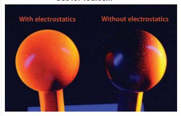
The black knob on the left was sprayed with fluorescent dye and with the electrostatic system turned on. However, the knob on the right was sprayed with the electrostatic system off. The spray coverage is so uneven that the back side of the knob remains untouched and is actually able to reflect the evenly-coated electrostatic knob.
